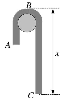
$$\left. \begin{array}{l} \ddot{x} - \frac{2g}{L}x = -g \\ x = \frac{2}{3}L \end{array} \right| \Rightarrow \ddot{x} = a = \frac{4g}{3} - g \Rightarrow \boxed{a = \frac{g}{3}}$$
